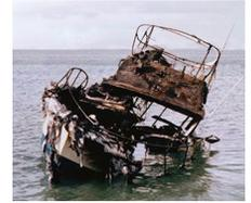
Gasoline vapors don't easily dissipate in closed engine compartments. Older gasoline powered boats often have brittle fuel hoses that can crack, leaving gas in the bilge after a fill-up. Practice safe refueling and better avoid fires like the one that happened in the photo above shortly after refueling.
